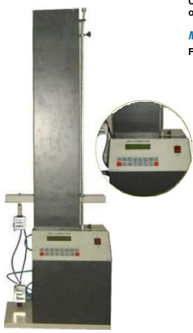
Compact & Elegant Table Top Design for strength testing of Yarn, Fabric, Lea, Elastomers, etc.
